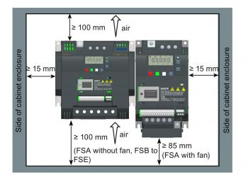
The inverter must be mounted vertically to a flat and non-combustible surface in an enclosed electrical operating area or a control cabinet.
