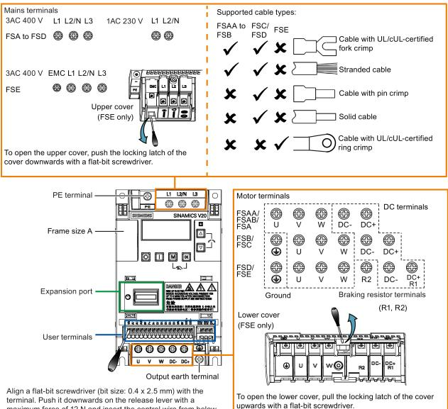
terminal. Push it downwards on the release lever with a maximum force of 12 N and insert the control wire from below.
